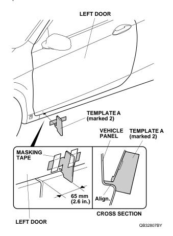
16. Using a felt-tip pen, mark the vehicle panel at the measurement shown.
