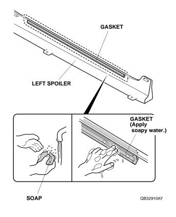
26. Secure the hook on the left spoiler to bracket B and align the gasket on the left spoiler with the rail. Insert the front end of the gasket into the rail first, then work rearward. Move the left spoiler up and down gently to make sure that the gasket is installed securely to the rail.
