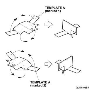
15. Place template A (marked 2) into position at the location shown. Align template A with the vehicle panel; lightly push down on the template, and attach it to the left door with masking tape. Make sure there is no gap between the template and the vehicle panel.
