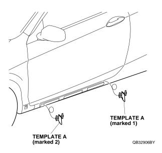
23. Using the palm of your hand, firmly press the rail against the vehicle panel for 30 seconds. Remove the mark you made using isopropyl alcohol on a shop towel.
